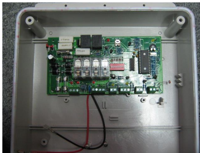
Figure 4: Point Lamp Photocell to the Side Gills of the Supplied Box for Ambient Light Detection.
